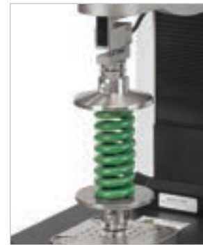
Compression spring testing
